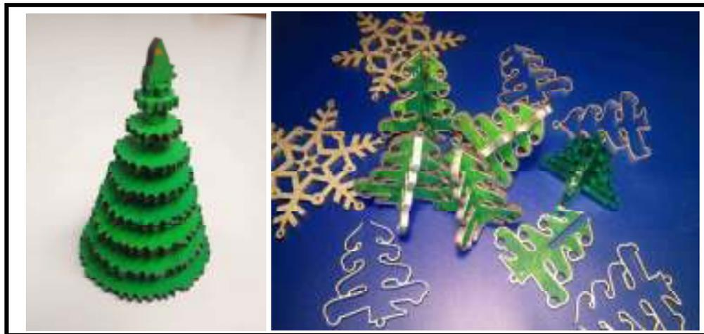
Slotty Trees is the perfect project to learn the process of making 3D objects from 2D shapes. A range of slotty products are shown here and they are all quickly made and assembled to provide that novelty aspect to your decoration.
